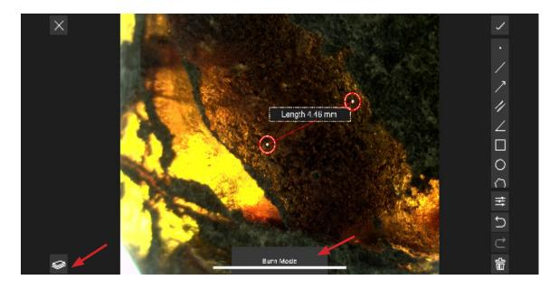
• When image is ready, tap the "<u>burn mode</u>" icon. This will "burn"/ save the measurements/annotations onto the image.
